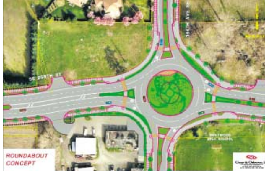
Roundabout design for S.E. 256th Street and 164th Ave. S.E.
